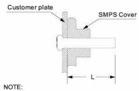
NOTE: Unit: mm ADJ:Output adjustable resistor Torque:M3, 0.5N • m Max TOL: ±1.00
